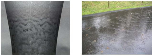
FIG. 1. (Color online) Waves in the Guinness and roll waves on a roadway in Craggaunowen, County Clare, Ireland. In the Guinness, the waves propagate downward and are superimposed on a circulatory motion whose origin appears to be due to buoyancy induced convection itself due to a lateral variation in void fraction. Photograph courtesy of Michael Manga [“Waves of bubbles in basaltic magmas and lavas,” J. Geophys. Res. 101 , 457 (1996) (Ref. 18)].
