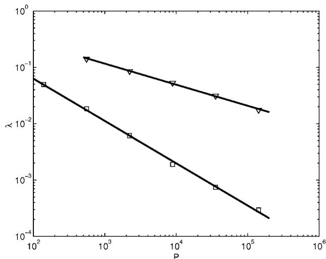
FIG. 9. Scaling of the exponential fits  $\lambda \exp(-\lambda n)$  to the  $m(n)$  curves. The triangles correspond to the stirring interval; the squares show the scaling of the long-time exponential decay rate. The fitted lines correspond to scalings of  $P^{-0.37}$  (triangles) and  $P^{-0.75}$  (squares).
