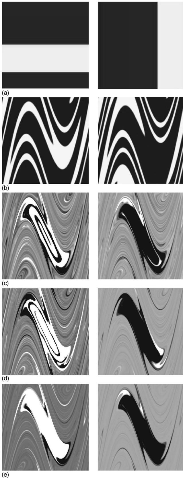
FIG. 6. Concentration density for initial condition 1 (left column) and condition 2 (right column). (a) Initial conditions, (b)  $n=2$ , (c)  $n=14$ , (d)  $n=24$ , (e)  $n=50$ . The highest concentration values in each picture are white, and lowest are black. Note the stirring effect within the island in the left column of (c) and (d).
