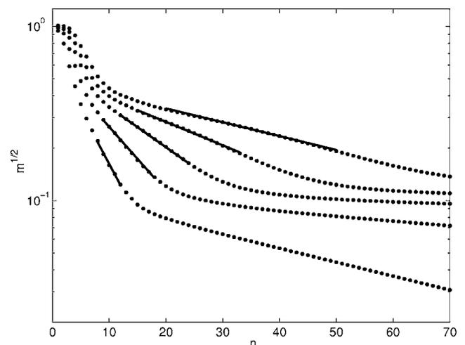
FIG. 8. Mixing measures  $m(n)$  for initial condition 1, for various Peclet numbers from 555 to  $1.42 \times 10^5$ . The Peclet number increases moving upwards among the curves. Exponential fits within the stirring interval are shown, the scaling of these fits is shown in Fig. 9.
