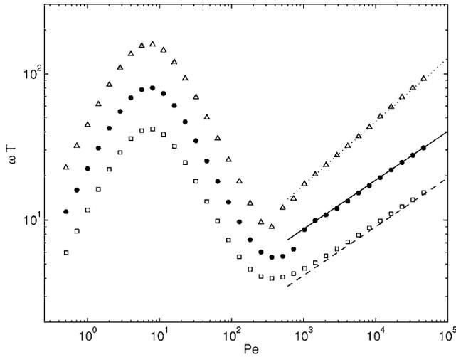
FIG. 4. Nondimensional mixing times as a function of Peclet number for  $\gamma=0.05$ . Asymptotic results are shown as lines, and numerical results as symbols for values of the mixing measure:  $M=0.3$  (dashed line, squares),  $M=0.1$  (solid line, points), and  $M=0.01$  (dotted line, triangles). The asymptotic result (23) is applied to the  $M=0.3$  and  $M=0.1$  cases, while the long-time version (25) is needed in the well-mixed  $M=0.01$  situation.
