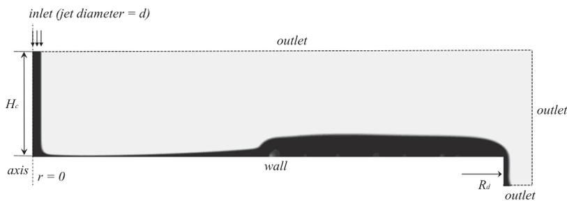
**FIG. 4.** Computational domain and boundary conditions.
