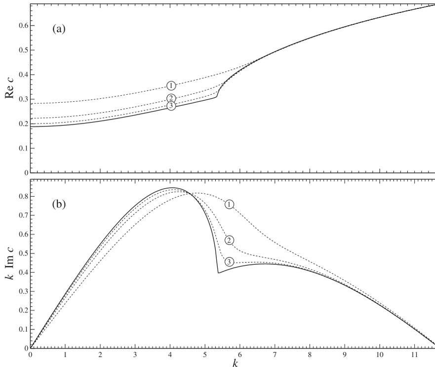
Fig. 3. The solution of the exact eigenvalue problem (20)–(22) (solid line) and that of the asymptotic problem (20)–(21), (23) with (1)  $D_a = 0.3$ , (2)  $D_a = 0.4$ , (3)  $D_a = 0.5$  (dotted lines). The Väisälä–Brunt frequency  $N$  and velocity  $V$  are given by (24)–(26) with  $\Delta_V = 0.12$  (thick flow).  $\text{Re } c$  is the phase speed of the disturbance and  $k \text{ Im } c$ , the growth rate.
