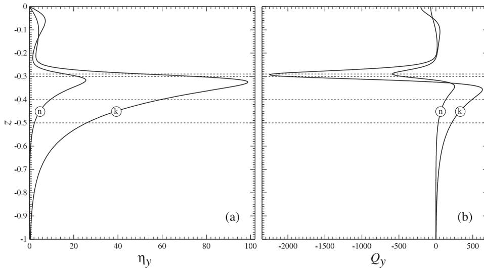
Fig. 2. The slope  $\eta_y(z)$  of isopycnal surfaces and the transverse gradient  $Q_y(z)$  of PV, for flows shown in Fig. 1. The labels (n) and (k) correspond to these in Fig. 1.
