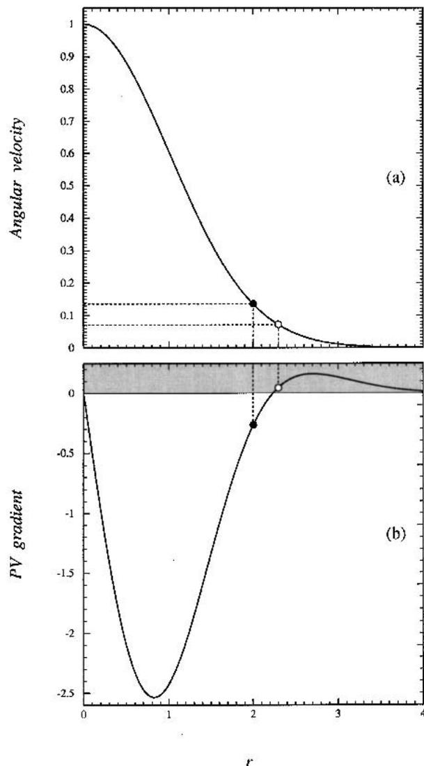
FIG. 3. The upper-layer (a) angular velocity  $(1/r)V_1(r)$  and (b) PV gradient  $Q_1'(r)$  for a Gaussian vortex. The region of positive  $Q_1'$  is shaded. Circles show the positions of the critical level: the open circle corresponds to  $S = 0$  (flat bottom), the filled circle corresponds to the case in which  $S$  and  $V_1$  are of the same sign. In the latter case, the critical level occurs in the region where  $V_1 Q_1' < 0$  (instability).
