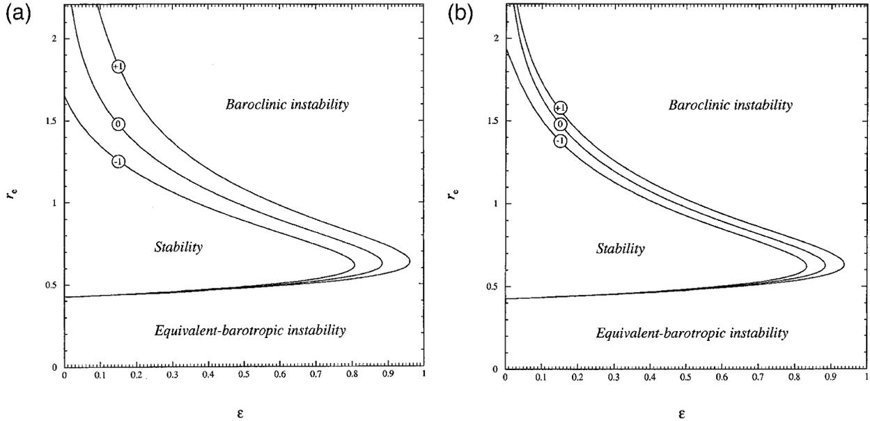
FIG. 1. The marginal stability curve for the Gaussian vortex over Gaussian topography, and the second azimuthal mode. Here  $\epsilon$  is the depth ratio of the ocean and  $r_e$  is the radius of the vortex [(8)]. The topography parameter is  $\delta = -0.1, 0$ , and  $0.1$ ; the corresponding curves are marked with  $-1, 0$ , and  $1$ , respectively. Curves are shown for (a)  $r_t = 2$  ( $r_t$  is the radius of the topographic feature) and (b)  $r_t = 1$ .
