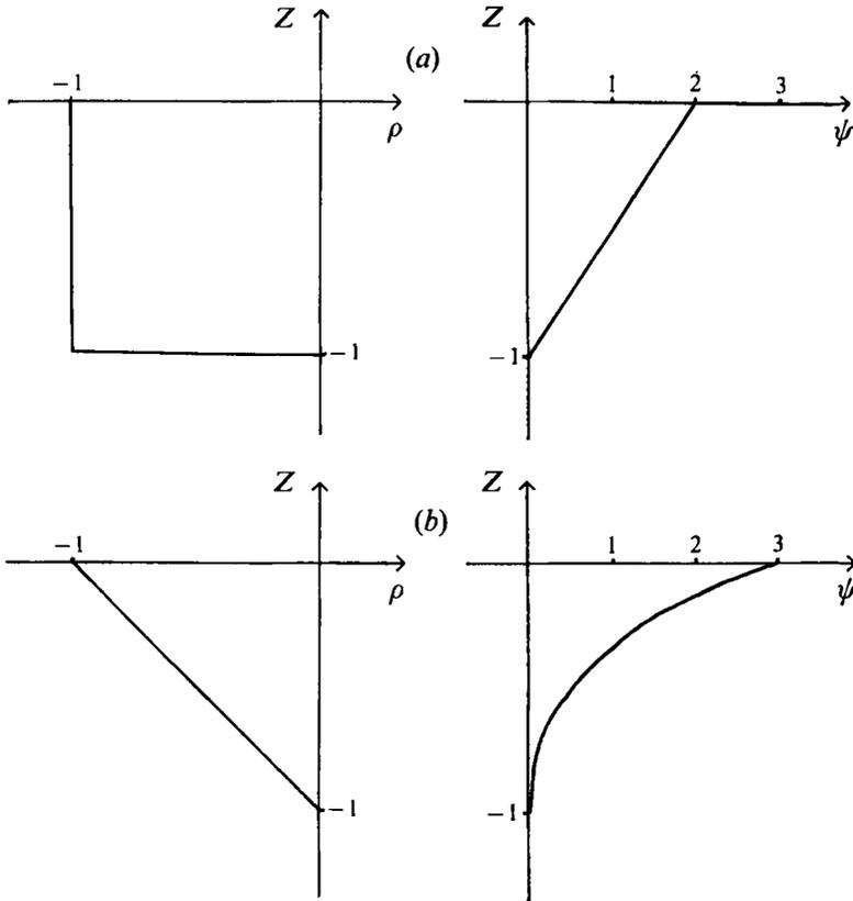
FIGURE 2. Two models of stratification for oceanic fronts.  $\psi$  describes vertical structure of the pressure field,  $\rho$  is the corresponding non-dimensional density variation: (a) two-layer model; (b) model with linear stratification of the upper layer.
