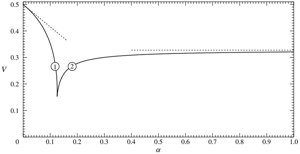
FIGURE 4. The dependence of the contact line’s velocity  $V$  on the parameter  $\alpha$  as determined by the boundary-value problem (4.6)–(4.11). The dotted lines show the asymptotic solutions (A 1), (A 12) ( $\alpha \rightarrow 0$ ) and (A 24) ( $\alpha \rightarrow \infty$ ). The solutions  $h(X)$  corresponding to points 1 and 2 are shown in figure 5.
