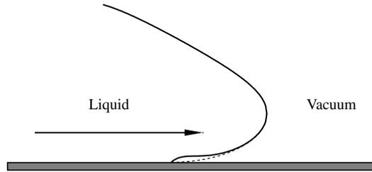
FIGURE 8. A flow over a plate (a schematic). The ‘microscopic’ contact angle differs significantly from  $180^\circ$ . The dotted line shows the ‘macroscopic’ structure of the free surface near the contact line.
