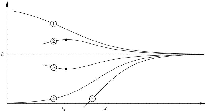
FIGURE 9. The five possible behaviours of the solution of the boundary-value problem (4.14) and (B 1). The dotted line indicates the limiting value of  $h(X)$  as  $X \rightarrow +\infty$  (see (B 1)). The black dots show the extrema (located at  $X = X_*$ ) of curves 2 and 3.
