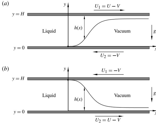
FIGURE 2. Couette flows with a free boundary, in the reference frame co-moving with the contact line: (a) flow of type A; (b) flow of type B.
