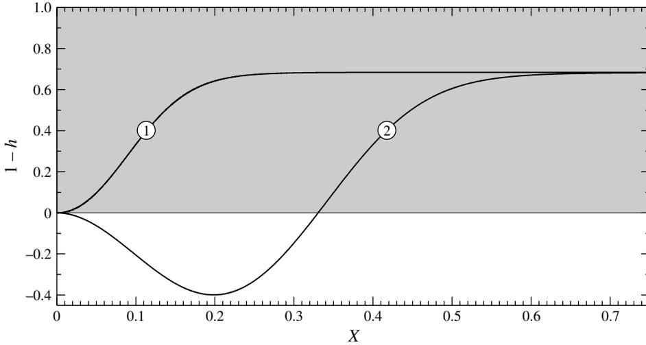
FIGURE 5. Examples of solutions of the boundary-value problem (4.6)–(4.11) corresponding to points indicated in figure 4: (1)  $\alpha = 0.1193$ ; (2)  $\alpha = 0.18$ . The region inside the channel is shaded. Observe that, in (2), the free boundary passes through the lower plate making this example physically meaningless.
