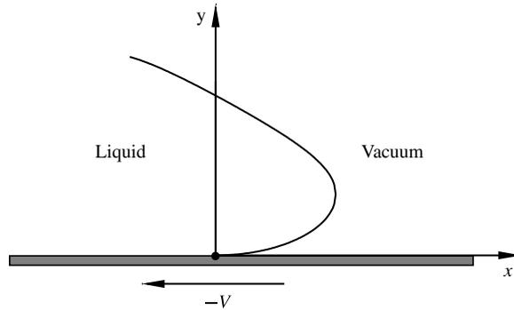
FIGURE 1. The setting of the local analysis by Benney & Timson (1980), in the reference frame co-moving with the contact line (shown by a black dot).
