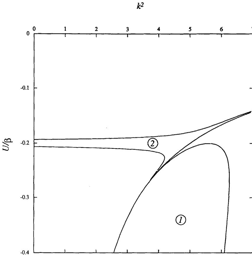
**Figure 2** The curve of marginal stability on the  $(k^2, U/\beta)$ -plane.  $h = 0.2$ ,  $\bar{v} = 0.001 U$ . (1) Phillips' instability; (2) the critical-level instability.
