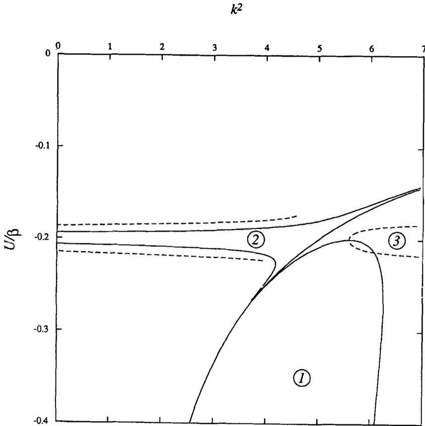
**Figure 3** The curve of marginal stability on the  $(k^2, U/\beta)$ -plane corrected for  $U \approx -\beta h$  by equation (36) (dashed line).  $h = 0.2$ ,  $\bar{v} = 0.001 U$ . (1) Phillip's instability; (2, 3) the critical-level instability.
