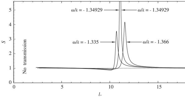
Figure 2. The dependence of the non-unitarity coefficient  $S$  [defined by (15)] on the meridional wavenumber  $l_-$  of the incident wave, for the Bickley jet (16), (17). Each curve is computed for a fixed value of the phase velocity  $\omega/k$  (indicated on the graph). Waves for which  $S > 1$  correspond to over-reflection.
