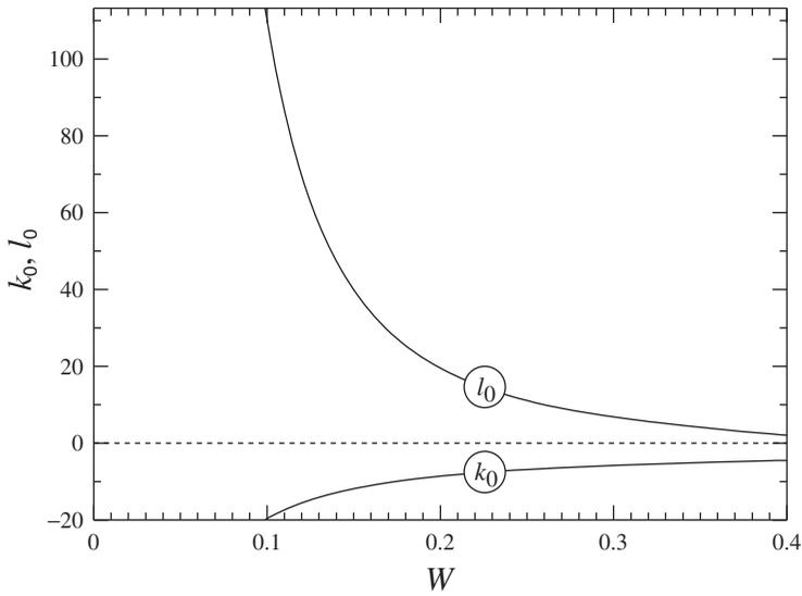
Figure 3. The wavevector  $(k_0, l_0)$  of the hyper-reflected wave versus the width  $W$  of the Bickley jet (16) with  $\Delta H = 1$ .
