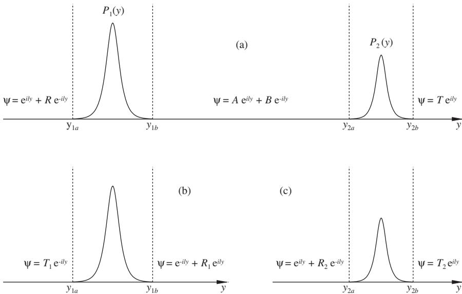
Figure 6. A schematic illustrating the scattering of waves by two potentials with compact, non-overlapping supports. Panels (b) and (c) illustrate wave scattering by the “individual” potentials  $P_1$  and  $P_2$ , panel (a) corresponds to the “global” scattering problem.
